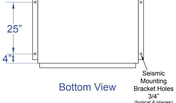
Per code requirements please leave 3" on each side of the cabinet including the back, and a 3 foot clearance in front.
